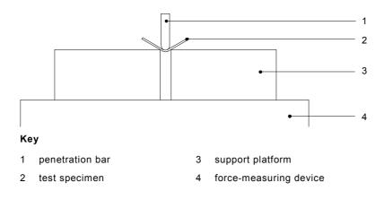
Figure 3 – Apparatus for measurement of stiffness
